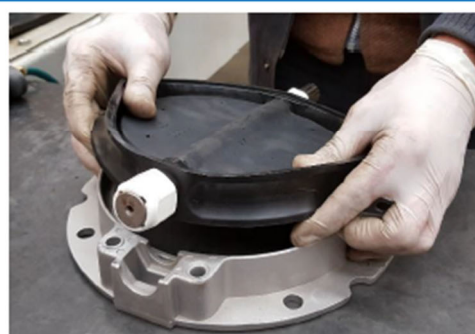
4- Fit the disc on the lower body of valve.
