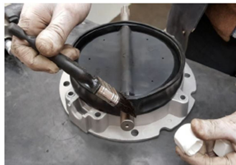
2- Apply oil to the two sides of disc's shaft.
