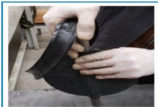
1- Fit the seal on the two sides of disc.
