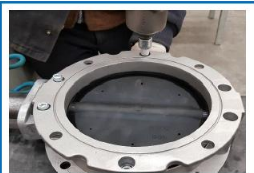
7- Fix bolts and nuts and tighten.
